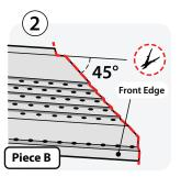
Cut the end of adjoining Piece B at 45-degrees. Repeat the 1/2 inch wide notch cut on the back wing and the 3/4 to 1 inch trim from the front edge. Pieces A & B should slightly overlap.
