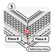
A completed outside corner should look like Image 3. For a tighter seal, place a screw through Piece B into Piece A to pull the pieces together.
