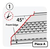
Cut the end of Piece A at 45-degrees. Next, cut a 1/2 inch wide notch from the back wing. Then, trim off 3/4 to 1 inch from the front edge in a straight line.
