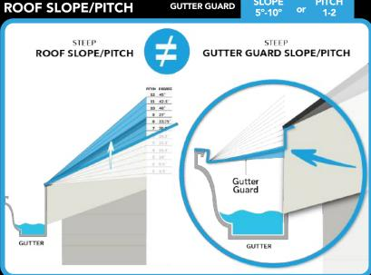
You will need to use one of the bending methods shown on p. 13 to achieve the recommended installation slope.
